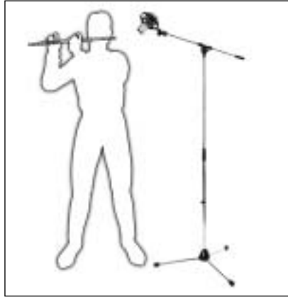
Fig. 8: Miking the flute with a single microphone.
